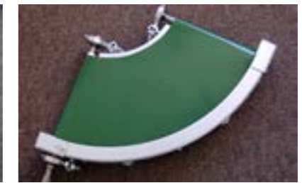
Curvebelt with a possibility for guidance control via ball bearings or buttons
