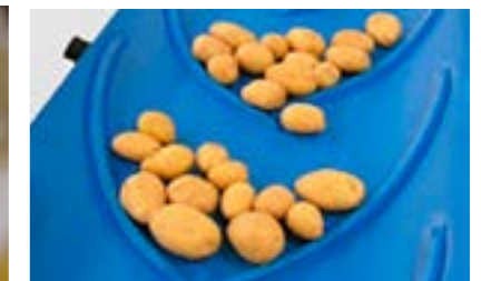
Special designed chevron belts for inclined transport of vegetables ie. potatoes
